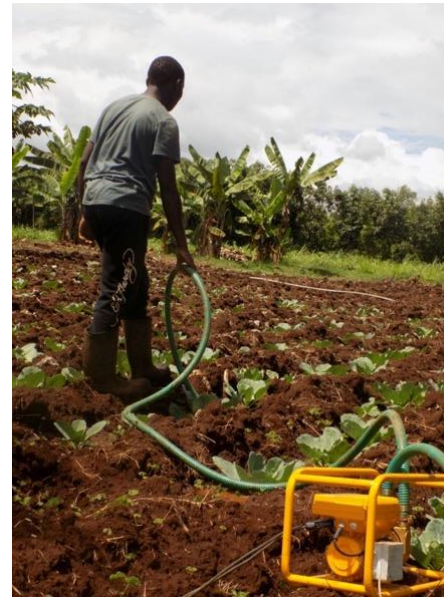
Installation on the surface if suction depth is < 7 meters
